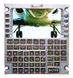
The crew can inspect the main landing gear condition by utilizing a bottom mounted cam era with the display on their CDU in the cockpit.
